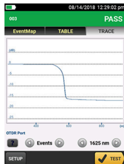
Splitter as seen on an OTDR trace
