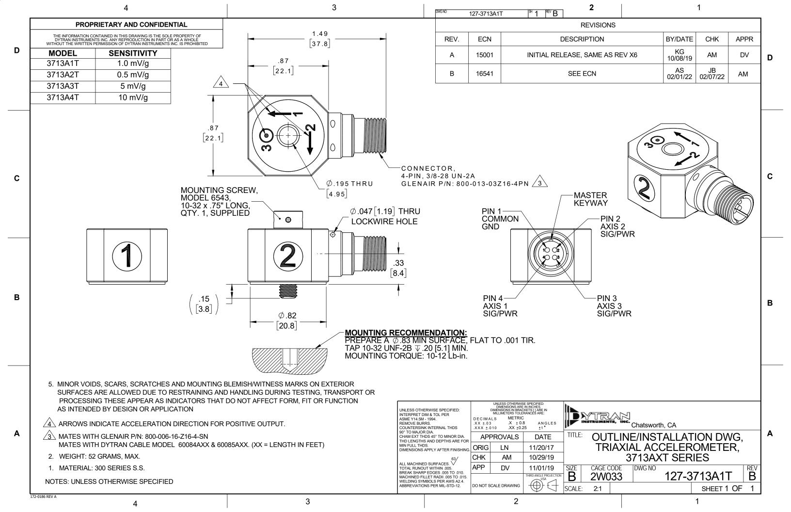
**Model Number** DOC NO PERFORMANCE SPECIFICATIONS 3713A3T PS3713A3T Triaxial Accelerometer, IEPE REV B, ECN 16541, 02/02/22
