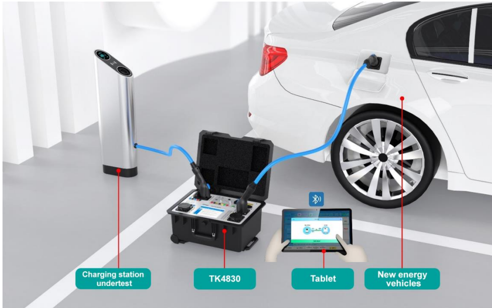
Test Method 1: Test with new energy vehicles as load
