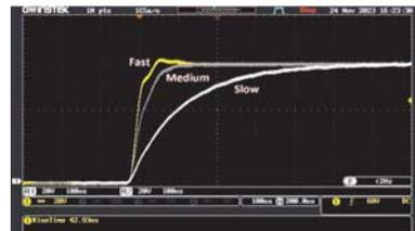
In order to meet the test requirements of different DUT output voltages, it is necessary to adjust the rise time of different output voltages. The ASR-6000 offers users up to three adjustable settings: typical values are fast (50 microseconds), medium (100 microseconds) and slow (300 microseconds). ASR-6000 is initially set to medium speed.
