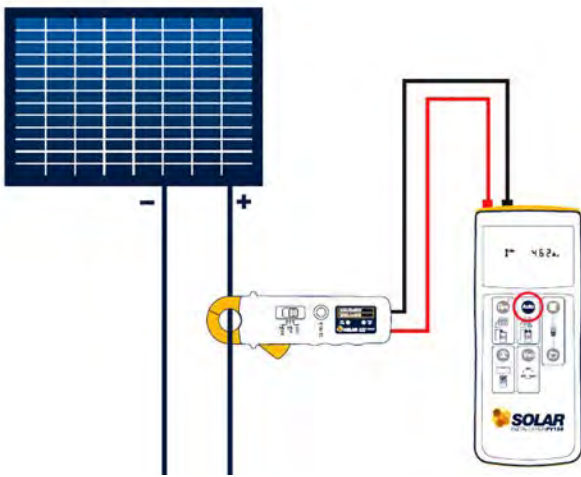
PV String Operation Current
