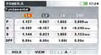
Power Measurements Summary (Fundamental)
