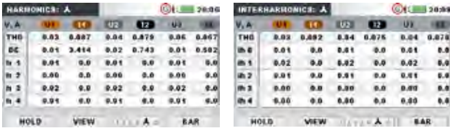
Harmonics and Interharmonics (METER) Screens
