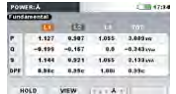
Power measurements summary (fundamental)
