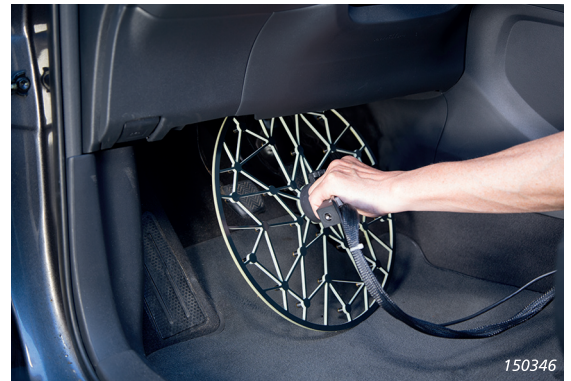
Fig. 4 Left: Array WA-1764-W-001 with reflective plate for use in beamforming measurements; Right: Without reflective plate for use in acoustic holography measurements
