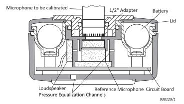
This microphone is optimized to have extremely high stability and independence of variations in static pressure and temperature around the 1 kHz calibration frequency. The result of this is a user-friendly calibrator where exact fitting of the microphone is not critical and the effects of changes in temperature and static pressure are negligible.
