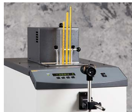
The 2019-DCB Liquid-in-Glass Thermometer Calibration Kit includes a carousel which holds up to 10 thermometers and an adapter tube which raises the bath fluid level to within 5–15 mm of the thermometers' readings. The 2069 Magnifier Scope mounts easily to the front of any Deep-Well Compact Bath to provide magnification of 8X or greater.
