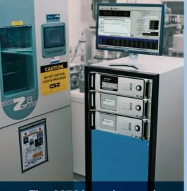
The 6270A can be used in system mode, allowing for multiple controllers to be operated through one front panel.
