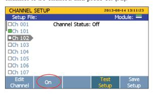
Press the **Edit Channel** soft key, set **Function** to Thermocouple, Thermistor, or PRT. Choose the appropriate parameters for the function selected. Configure additional channels. Press **Back** when finished.
