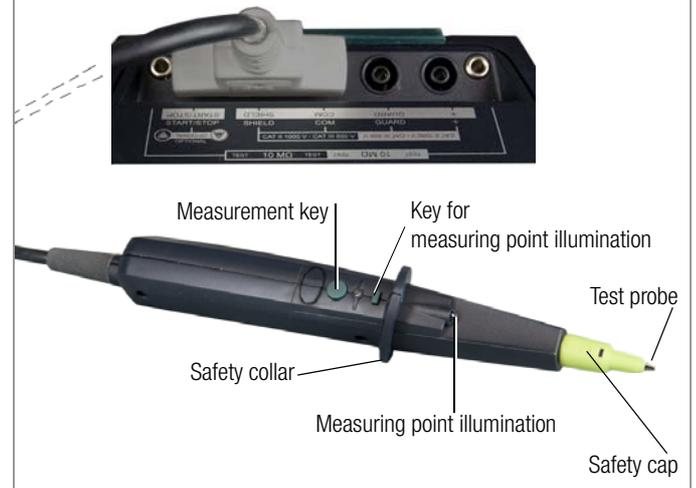
The test probe with integrated control module allows for remote triggering in areas with difficult access or in situations which require your full attention. Poorly lit measuring points can be illuminated with the integrated test probe lighting. The connection cable is shielded from interfering influences.
