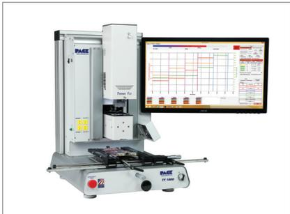
**TF 1800 BGA/SMT Rework Station with Inductive-Convection Technology**
