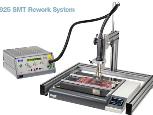
The ST925 combines three popular PACE products together into one convenient, low-cost SMT Rework System. The system is comprised of the **ST325 Programmable Convective/Hot Air Rework Station**, the **PH100 Low Profile Infrared Preheater**, and **ST500A Z-Axis Platform**. Together, the system provides a powerful 575 Watt convective top-side heater plus a 1600 Watt IR bottom-side preheater which allows operators to safely rework PCBs.
