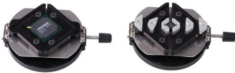
Two (2) removable and adjustable Component Nests are provided for perfect centering of components, in preparation for vacuum pick-up/placement. In addition, a Small Parts Nest (not shown) is provided for components less than 5mm sq.
