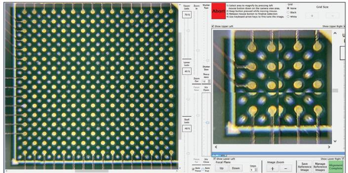
A high definition Vision Overlay System uses bright white LEDs with independent intensity control to provide precise distinction of pads and solder ball or leads.
