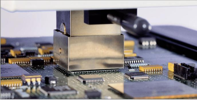
Newly designed reflow head provides smooth, precise movement with no drift, allowing for repeatable and accurate placement.
