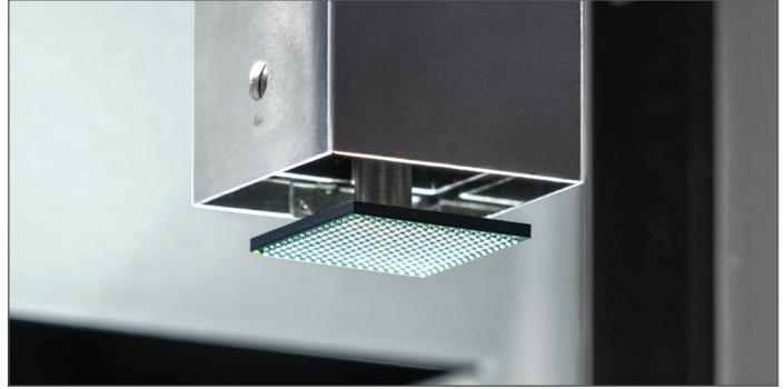
New Vacuum Pick design is more robust, utilizes an optical sensor, is counterweight balanced, and uses precision high temperature linear ball bearings for the highest sensitivity in placement and pick-up.
