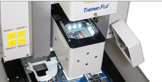
An automated Vision Overlay System uses a dichroic beam-splitting prism, high intensity LEDs, and new high definition 1080p camera to easily align any component.
