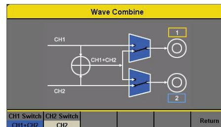
Create complex waveforms by internally adding each channel's waveform and outputting the combined waveform on channel 1 or 2.
