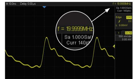
Built-in arbitrary waveform at 20 MHz, 300 MSa/s
