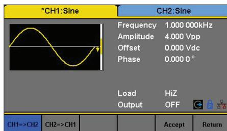
With the push of a button, all waveform parameters can be quickly copied between channels. Phase between channels can be adjusted.
