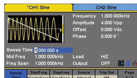
Perform linear or log sweep functions with up or down directional control. The sweep source can be set to internal, external, or manual.
