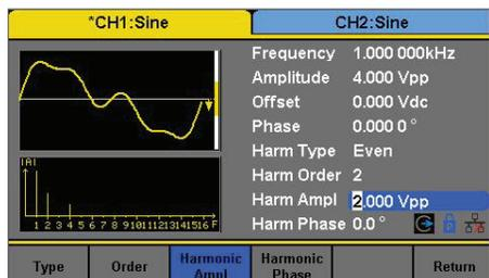
Quickly output harmonics up to the 16th order with independent amplitude and phase settings.
