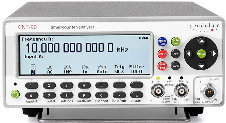
The Pendulum CNT-90 timer/counter/analyzer is an ultimate tool for measurement, analysis and calibration of Frequency, Time Interval or Phase. The CNT-90 is a high-performance counter with a fast measurement speed to 250,000 measurements/s, and time interval measurement resolution to 100 ps. The CNT-90 offers ease-of-use including graphical display and improved display and improved control over measurement at an outstanding price.
