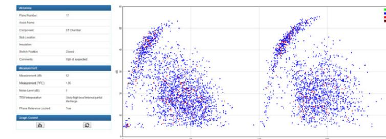
Example of internal void PD measured using the TEV sensor. Asset information can be transferred and sent to EA Technology or your in house PD experts for review.
