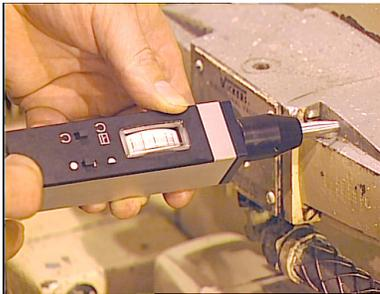
**The UL101 Receiver shown here with 1-inch solid probe testing solenoid valves for bypass leak**
