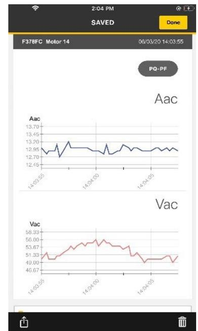
Data gathered by Fluke Connect can pinpoint elusive intermittent faults. Data collected over regular intervals can be used to spot small changes before they grow into major problems.
