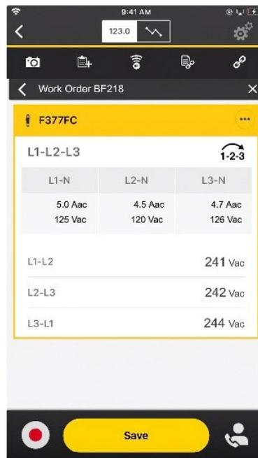
Fluke Connect pulls all data related to three-phase measurements including phase rotation and presents the full set of data for analysis at a glance.
