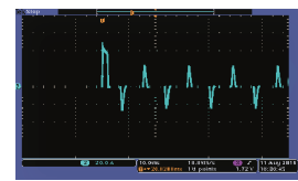
Inrush Current for 90° Start Angle
