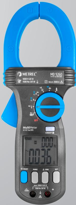
The MD 9260 is the first Metrel instrument to support measurements up to 1500 V DC with CAT III safety. Its voltage range and safety make it useful in highly demanding environments like solar power plants, wind power plants, or other high power environment using DC current. It has 2000 A AC / DC current range and can additionally measure resistance, capacitance, frequency and temperature – in short a well-rounded multimeter-style tool for use in power applications.
