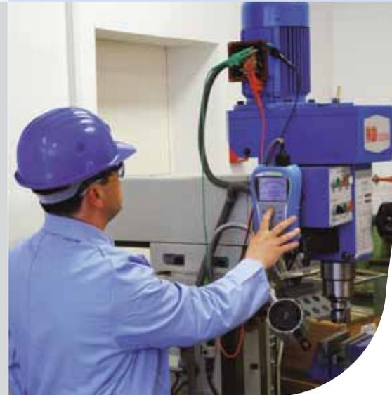
The MI 3121H Smartec 2,5 kV Insulation / Continuity is the portable measuring instrument for complete diagnostic testing of insulation and continuity measurements. Due to insulation resistance measurement with the test voltages up to 2.5 kV (measuring range is up to 100 G $\Omega$ ) and calculation of PI and DAR indexes the instrument is ideally suited for testing insulation of cable lines, current and voltage transformers, electric motors, etc.
