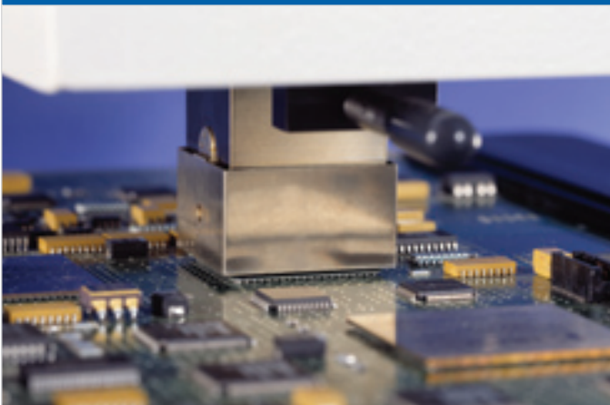
Nozzle lowering over PBGA for reflow
