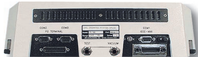
PG Platform - Rear Connections
