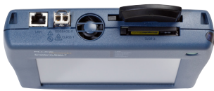
Top interfaces - 10/100/Gigabit twisted pair copper port, Gigabit Fiber SFP transceiver, Compact Flash memory card, and 802.11a/b/g WLAN PCMCIA card.
